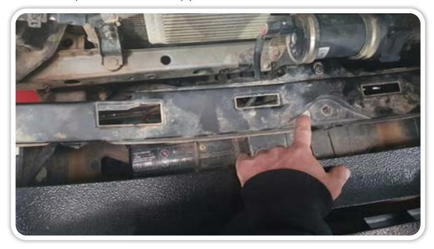
**1.6.** Unbolt the right side horn (drivers perspective) from the upper support panel. Horn will be remounted to the cooler bracket. Keep the factory M8 bolt for use later.
