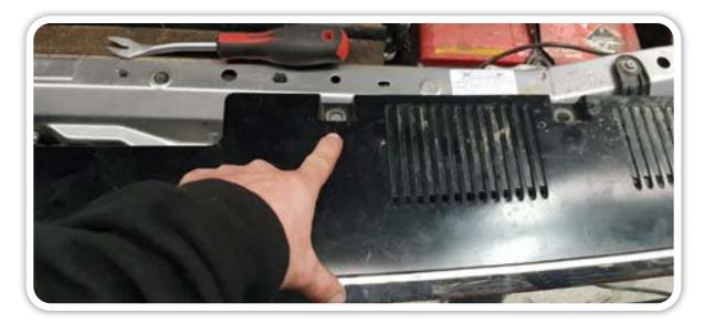
**1.3.** Ensure all bolts are removed, they are located not only on the radiator support bar but also on each side headlight.
